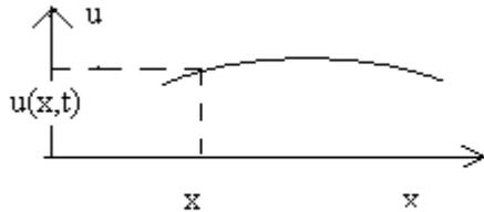
$$\mu \frac{\partial^2 u}{\partial t^2} = T \frac{\partial^2 u}{\partial x^2}$$
