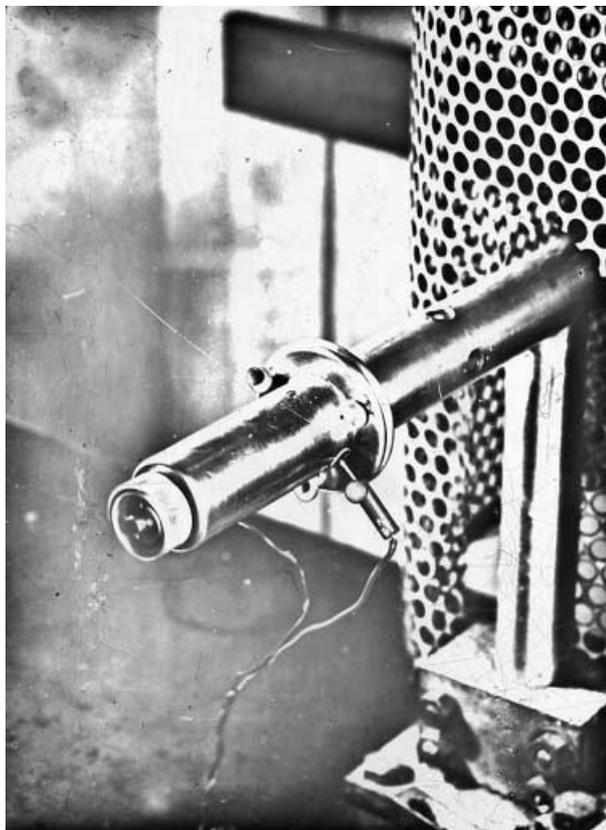
**Fig. 2.** Prototype model of Ehrenberg-Spear fine-focus X-ray tube used in early muscle work (diameter of tube is approximately  $3.5\ \text{cm}$ ). Anode connection is inside safety shield, at 40 kV.
