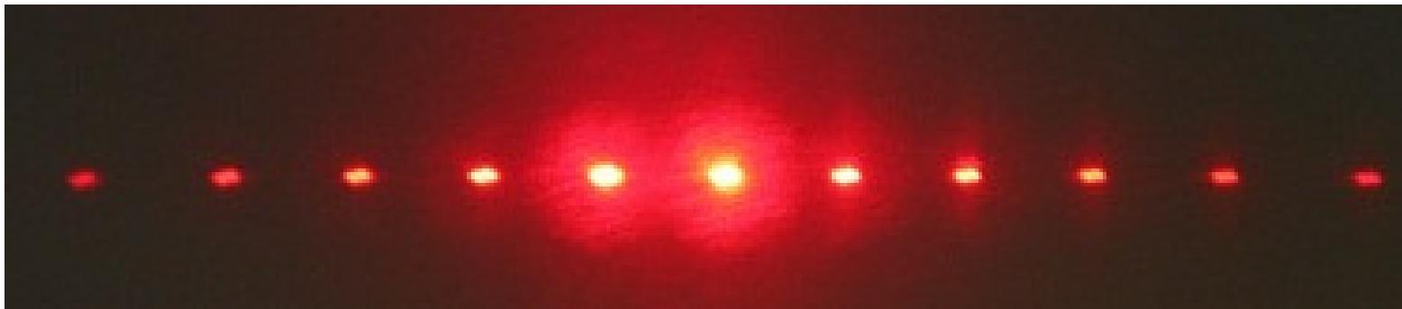
A beam of helium-neon laser is diffracted to each side in multiple orders.
