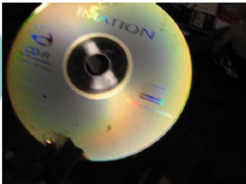
**1: Scratch the label surface of the CD to begin especially with painted labels (Blank CDs work best).**
