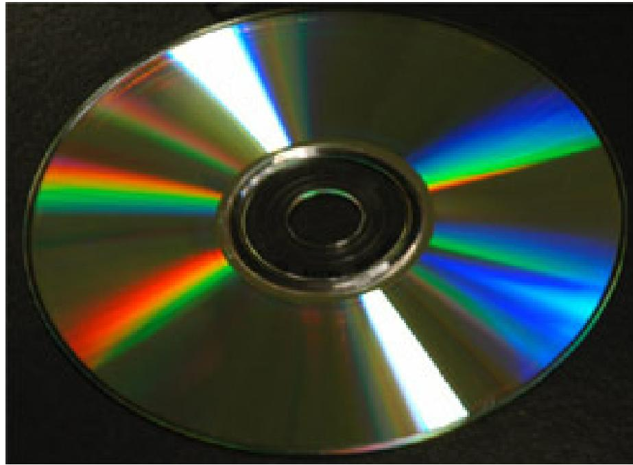
The tracks of a compact disc act as a diffraction grating, producing a separation of the colors of white light.
