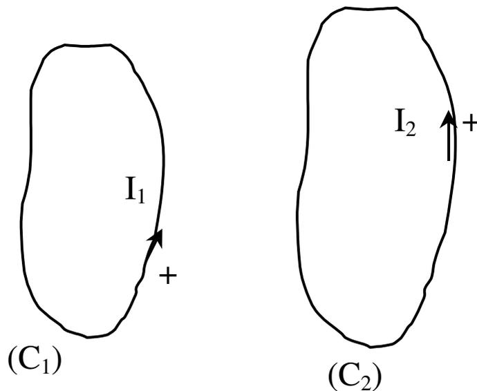
$$\Phi_1 = L_1 I_1 + M I_2 \quad \text{et} \quad \Phi_2 = L_2 I_2 + M I_1$$
